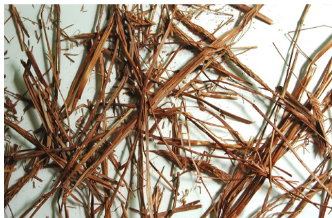
(7) Well-preserved straw of a 700-year-old straw-clay filling from 1298, Limburg [Lit. 3].
